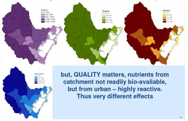
Considering the Total Catchment Model, the larger catchments produce the most "stuff". The "stuff" from the upper catchment is different from the "stuff" from the lower catchment. They come down into the lake by rivers and creeks. In the urban catchments the runoff from the roads. The nutrients are attached to the sediments. The total nitrogen from the road is quiet different from those from the upper catchment.
